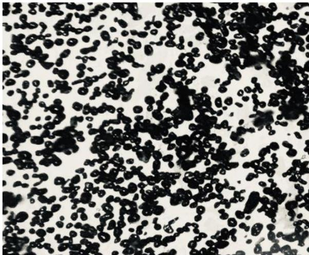
Microscopic pictures of **EcoGrafi** spherical graphite, with the round shape of the individual particles clearly visible, as well as the uniform particle size distribution in the sample, both key criteria for high quality spherical graphite.
