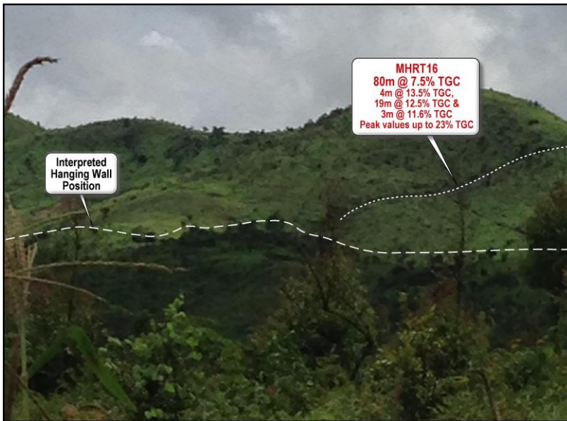
Figure 3: View from the eastern zone from Hole MHRC019 looking west, showing the western zone mineralisation and interpreted contact position (hangingwall) of the graphite mineralisation.
