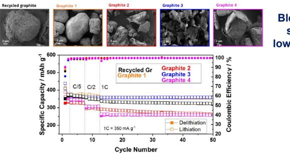
Electrode contains: 95% recycled graphite(+3% SBR, 1% CMC, 1% C45)
