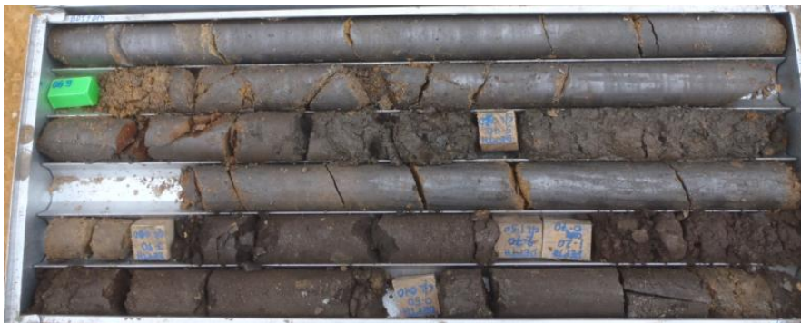
Figure 2: MHDD001 showing the graphite mineralisation in a core tray. Flake graphite is observed throughout the entire interval.
