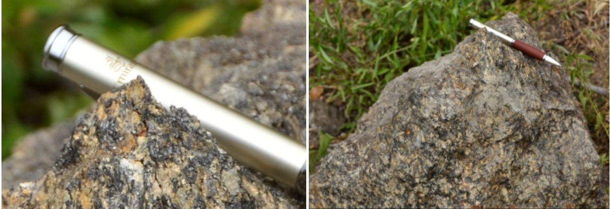
Pictured: Outcropping gneiss with large flake graphite (dark grey minerals) at Merelani-Arusha project.
